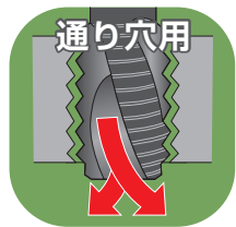
切屑の排出方向が 前方 Chip discharge direction is forward
