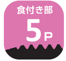
先端食付き部の ねじ山数 Number of threads on tip chamfer
